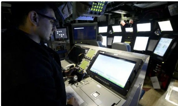
Left: a Sailor mans the photonics mast controller aboard a Virginia-class submarine (Source: Reddit). Right: L3Harris integrated submarine mast system diagram (Source: L3Harris).
